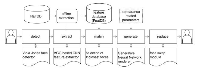
Fig. 1. Block diagram of our deidentification pipeline. The procedure uses a generative neural network to generate synthetic faces that can be used for deidentification. Each generated face is a combination of k identities from the gallery data that are closest (i.e., most similar in the feature space) to the input face.
